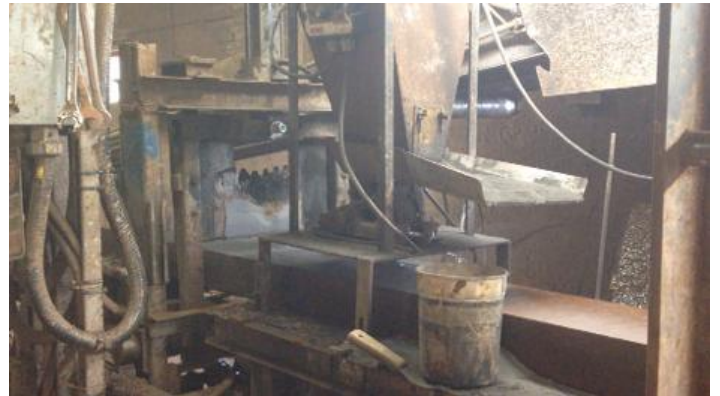
CUTTING SECTION of BRICK
